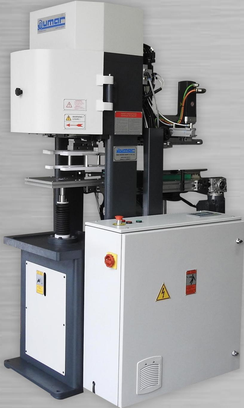
Fully automatic single head can seaming machine is designed for seaming of round tin, aluminum or composite cans. Different versions are available according to can size and seam type i.e. double or triple seam. Freestanding fully automatic machine is with its own conveyor.
